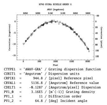
**Fig. 4.** KPNO Hydra Fiber Bench Spectrograph using an echelle grating in 11<sup>th</sup> order with a 2K CCD.
