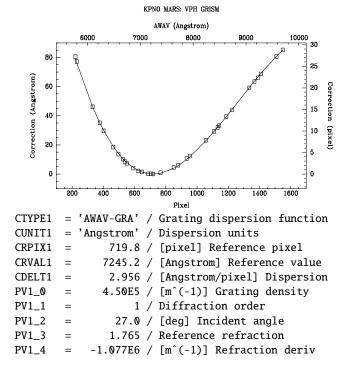
**Fig. 5.** KPNO MARS spectrograph with a 450 lines/mm volume phase holographic grism and a 2K CCD.
