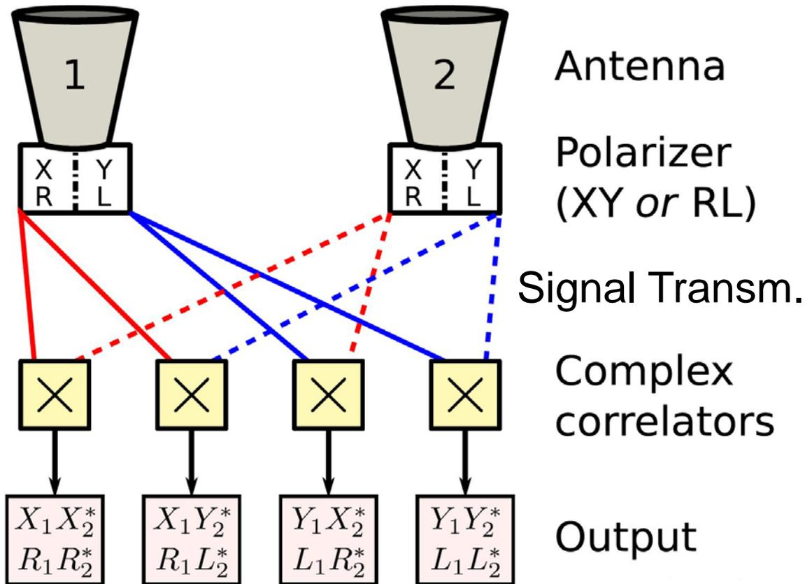
Two antennas, each with two differently polarized outputs, produce four complex correlations.
