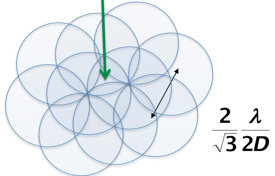
Most efficient coverage with minimal non-uniformity (centers on equilateral triangles). Preferred!
