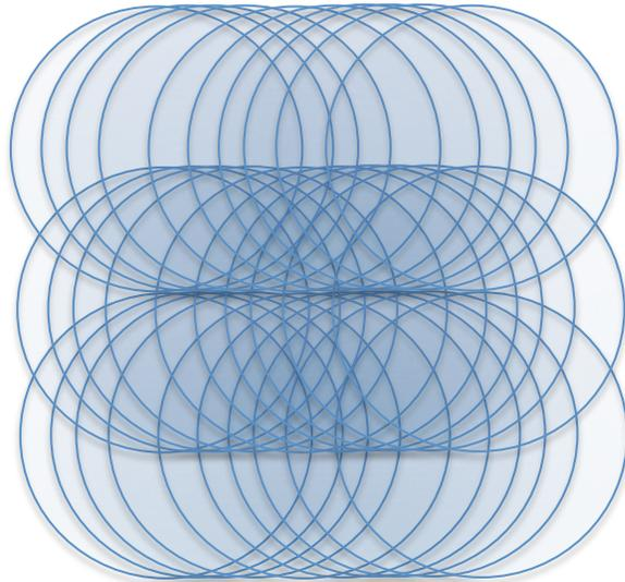
Antenna scan does not stop, fast dumping of data, influences the primary beam shape, produces lots of data but reduces overhead
