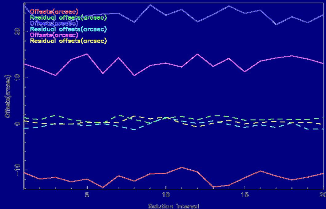
Continuous lines: Typical antenna pointing offsets for VLA as a function of time (Mean between +/- 25" and RMS of 5").
