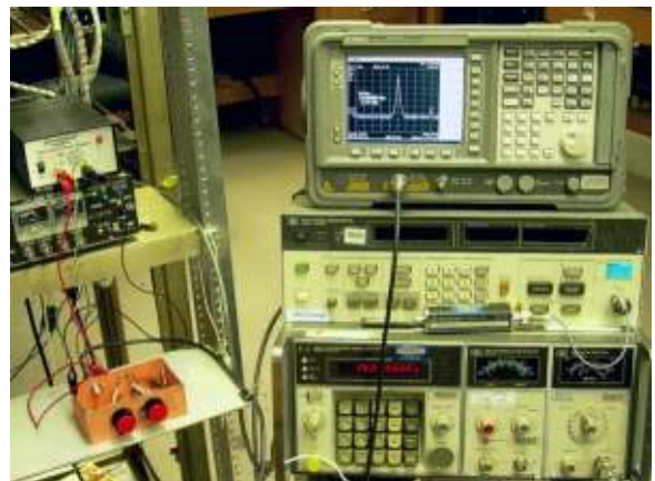
Some of the test equipment at the VLA observatory for testing the low band receiver upconverters (for 74, 196 and 327MHz receivers). The Agilent E4406 spectrum analyzer was used to test the hetrodyne VFO for spectral purity and phase noise.
