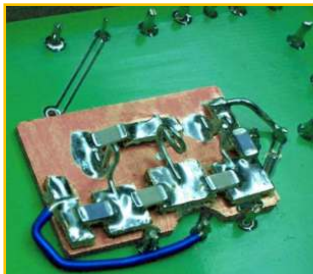
FIG. 17 – The temporary 1090 MHz High Pass Filter added to the PCB.
