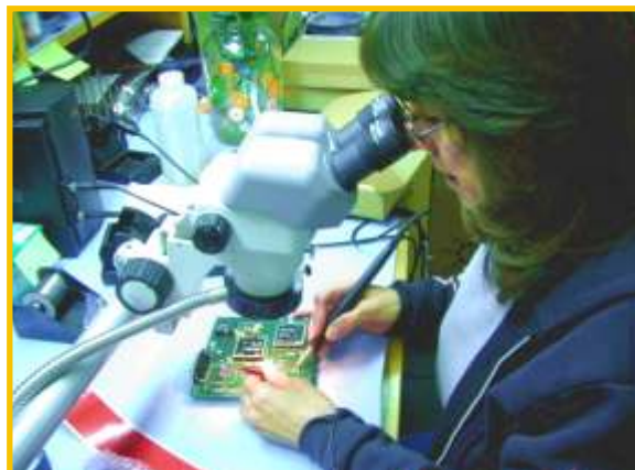
Fig. 8 – Connie Angel, one of the professional assemblers at the VLA observatory, solders surface mount components onto a board with tweezers and a soldering iron. The board is part of a new radio telescope (called ALMA) being built in Chile.
