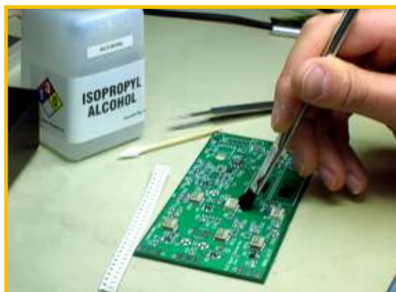
Fig. 9 – Clean solder connections with a hobby brush and alcohol. This keeps the board clean and free of corrosive rosin, whether building Manhattan or a PCB.
