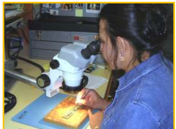
Fig. 23 –After manually applying the paste, Mary Ellen Chavez places the SM components on the board with tweezers and microscope prior to reflow soldering.
