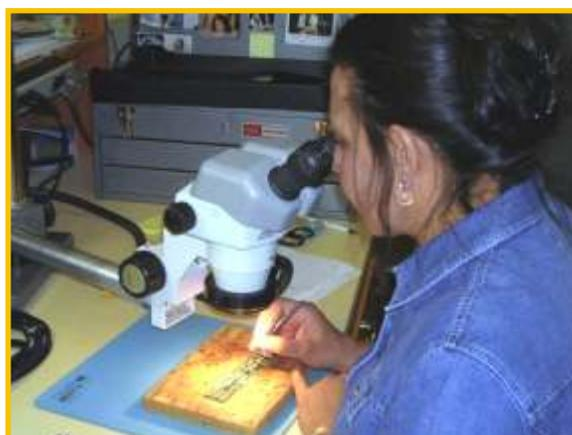
Fig. 23 –After manually applying the paste, Mary Ellen Chavez places the SM components on the board with tweezers and microscope prior to reflow soldering.
