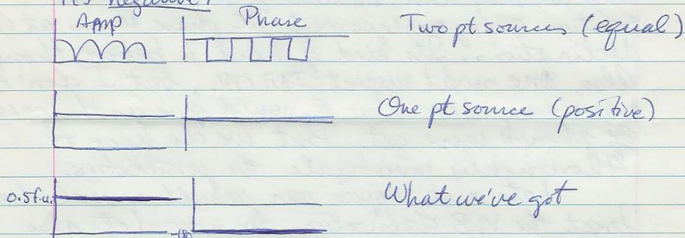
I'm sort of worried that we have a calibration error of  $180^\circ$ , but somehow I can't bring myself to believe that's behind our results. It's not a random calibration error - after all we have 6 independent baselines on 2 days, and all the phases are  $\sim 180^\circ$  (except in the hills) and the amplitudes hang in there at 0.5 f.u. (with a possible slight decline to 0.45 f.u. when the projected baseline gets longest).
