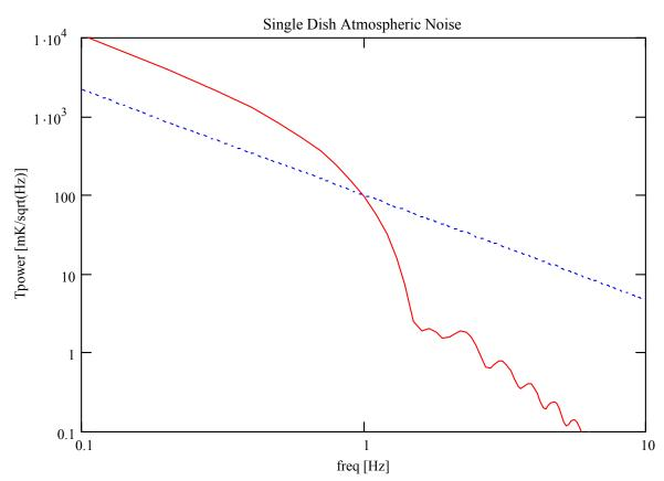
Calculation of the atmospheric noise for a single dish staring at the sky using the same assumptions as ALMA Memo 422; 250 micron RMS noise from the 300 m baseline phase monitor and a conversion of 20mK/micron from delay to sky brightness.
