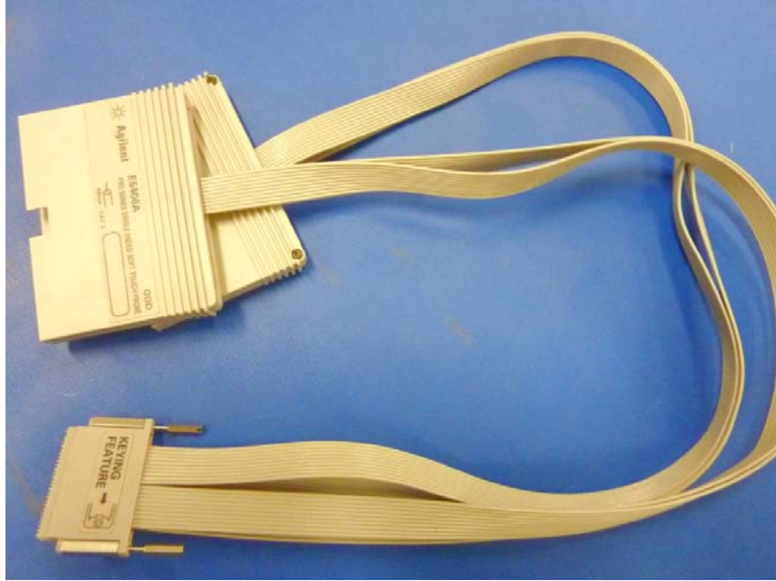
Figure 6-20 Agilent soft-touch E5406A pod assembly.
