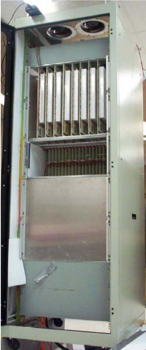
Figure 15 (Right) Close-up of heat-producing boards, heatsinks, and fans in the thermal test rack. (Below) Thermal test rack.
