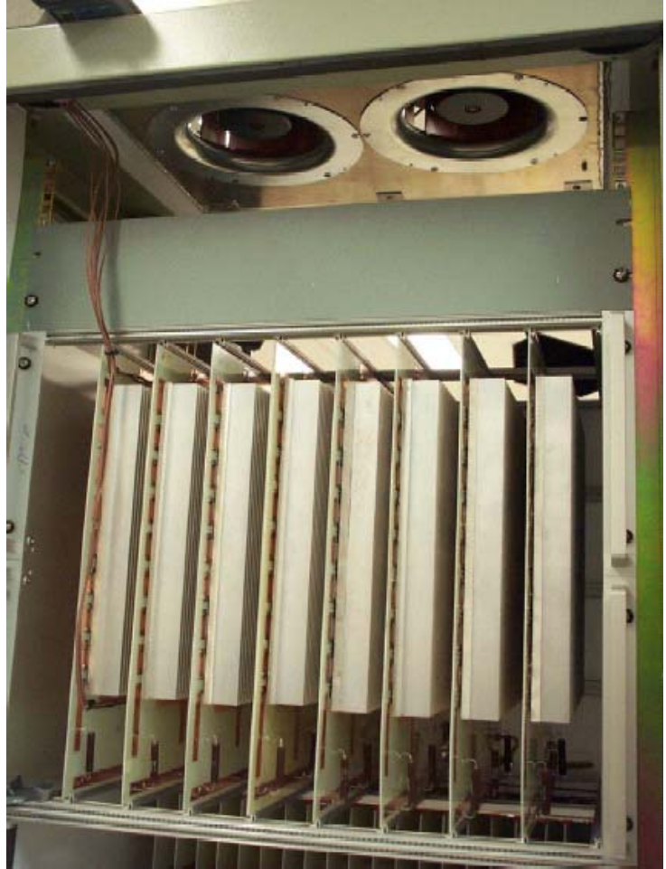
Figure 15 (Right) Close-up of heat-producing boards, heatsinks, and fans in the thermal test rack. (Below) Thermal test rack.
