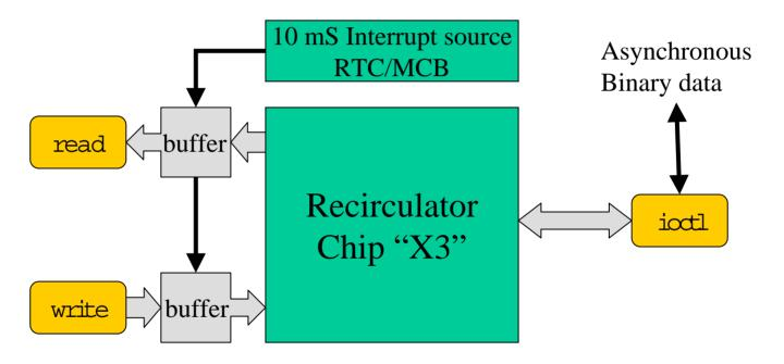
Buffer contains Timecodes and HM signal stats in binary, updated (pushed, pulled) every 10 milliseconds.
