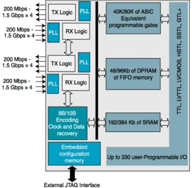
Cypress Semiconductor "Frequency Agile" PSI with 4 or eight serial channels operating from 0.2 to 1.5 Gbps. http://www.cypress.com/psi/index.html
