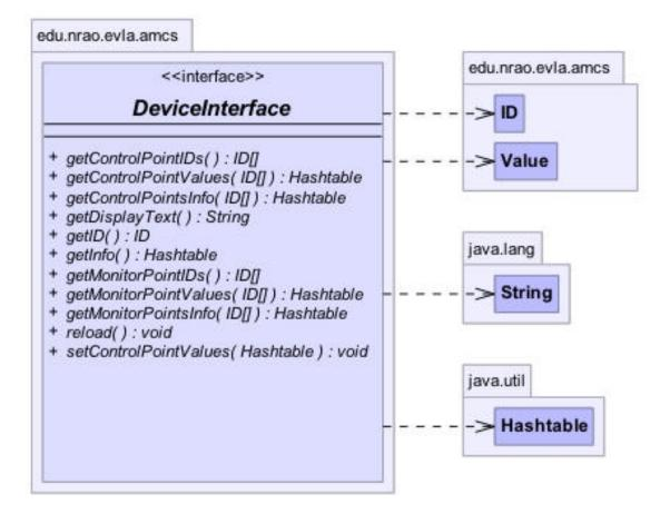
The DeviceInterface will not be used for normal operation of the system because it would mean that raw monitor and control data would be flowing across the system to the operations program. Since operations must be maintained on a generic level this will not work.
