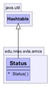
Status is a class that is used to represent any kind of status from a simple Boolean go/nogo to complex structures containing state along with possible amplifying information such as fault analysis or corrective maintenance advise.
