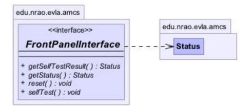
The FrontPanelInterface does not do much by itself except specify a minimal set of methods that all Devices must provide. It is the intent that Specific Devices must extend the FrontPanelInterface to provide the functionality needed to fully operate them.
