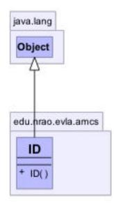
The ID class represents an identifier for every Device, MonitorPoint and ControlPoint in the system. ID was made a class instead of a string or integer to allow more flexibility.
