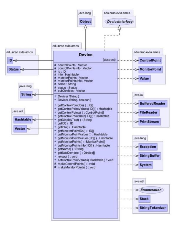
The Device base class must be extended by each of the component classes (i.e. the ElevationServo class). This makes the ElevationServo everything that a Device is but with additional characteristics specific to that of an Elevation Servo.
