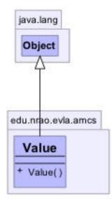
Value is a class that provides a means to communicate data across module boundaries without having to use specific data types.
