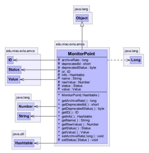
Most MonitorPoints will be updated by their Device, either periodically or asynchronously when the MonitorPoint is requested. It is possible, however, that some MPs and CPs could contain their own Thread. In those cases, they will be compiled into the Device and not instantiated at run-time as described next.
