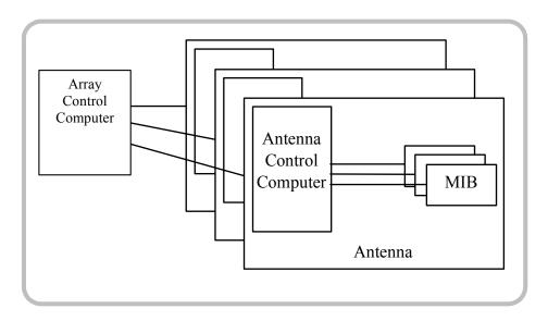
Whether the Antenna Control Computer resides in the antenna itself as shown above or resides in the Control Building, its functionality will remain about the same. The Module Interface Boards (MIB) operate specific antenna hardware, the Antenna Control Computers operate the MIBs and the Array Control Computer operates the Antenna Control Computers.
