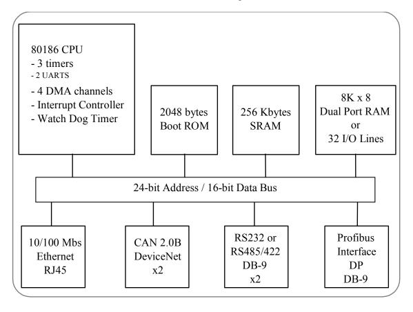
The MIB provides the interface between the Antenna Control Computer software and the antenna hardware. It will communicate with the Antenna Control Computer through the Ethernet port and with the antenna devices through one or more of its various other ports. This has the effect of converting the differing interface requirements of the various antenna devices into one interface type (Ethernet) for communications with the Antenna Control Computer.
