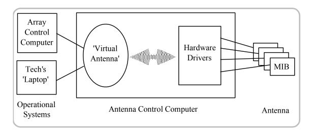
The Antenna Control Computer is the computer 'closest' to the antenna hardware itself. It presents a virtual representation of the antenna hardware to the rest of the AMCS and configures the antenna hardware to the state desired. It directly monitors and controls one antenna.
