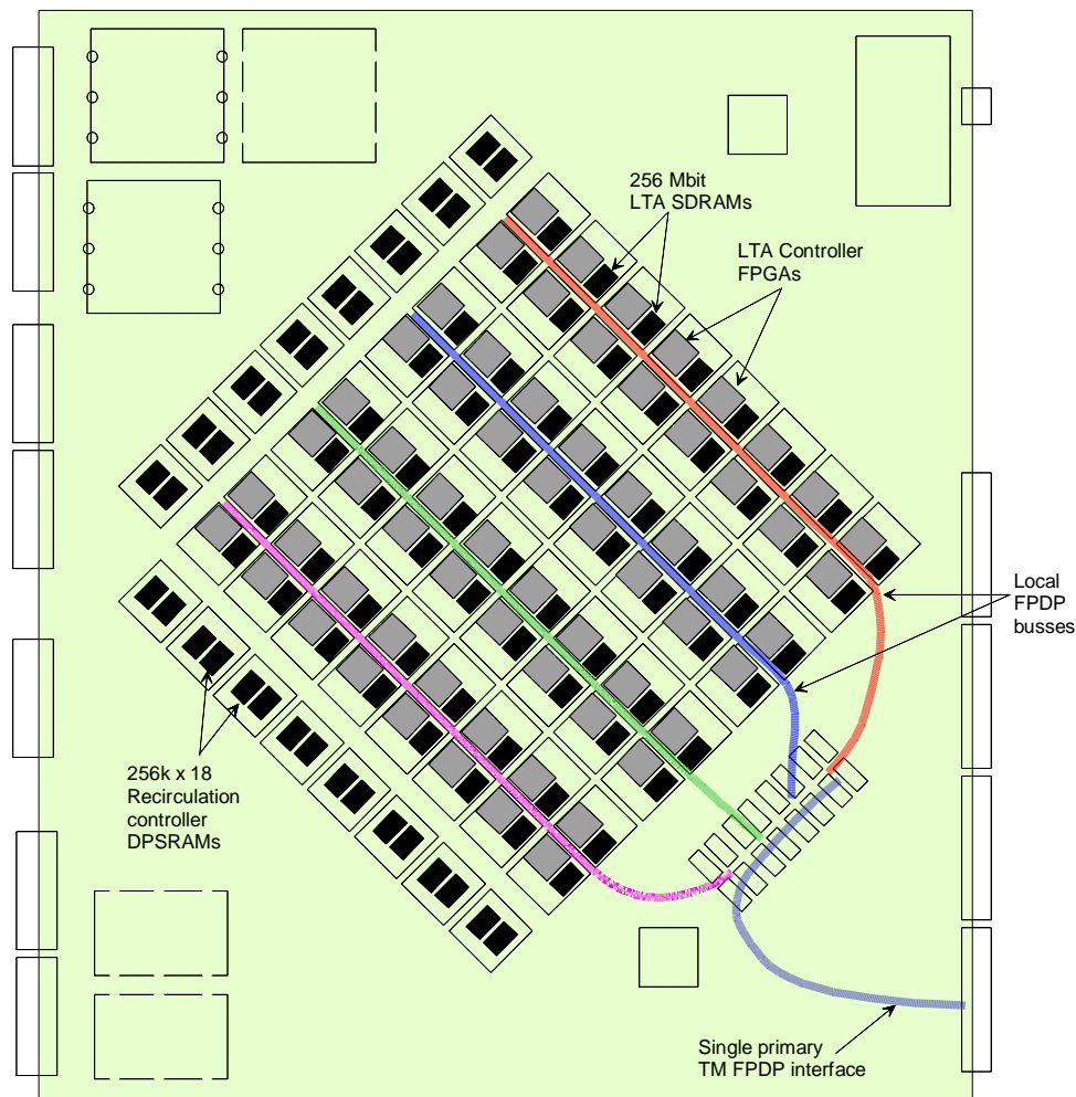
Figure 4-47 Local FPDP bus routing with one active external FPDP transmit interface. The FPDP Scheduler enables only one correlator chip and one set of FPDP drivers at a time. With this arrangement and a 100 Mbytes/sec FPDP interface, all lags from all correlator chips can be dumped about every 11 milliseconds. This should be more than adequate for most applications.
