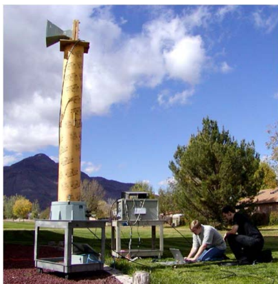
Figure 1. Basic AUT Tower using Sono-tube™ and wood. (Source Tower is of similar construction)
