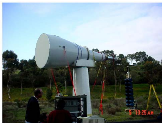
Figure 2. L-Band test setup conducted at Composite Optics, Inc. in San Diego, CA. The foam tower depicted here represents the type of construction that will be used on the OATR.
