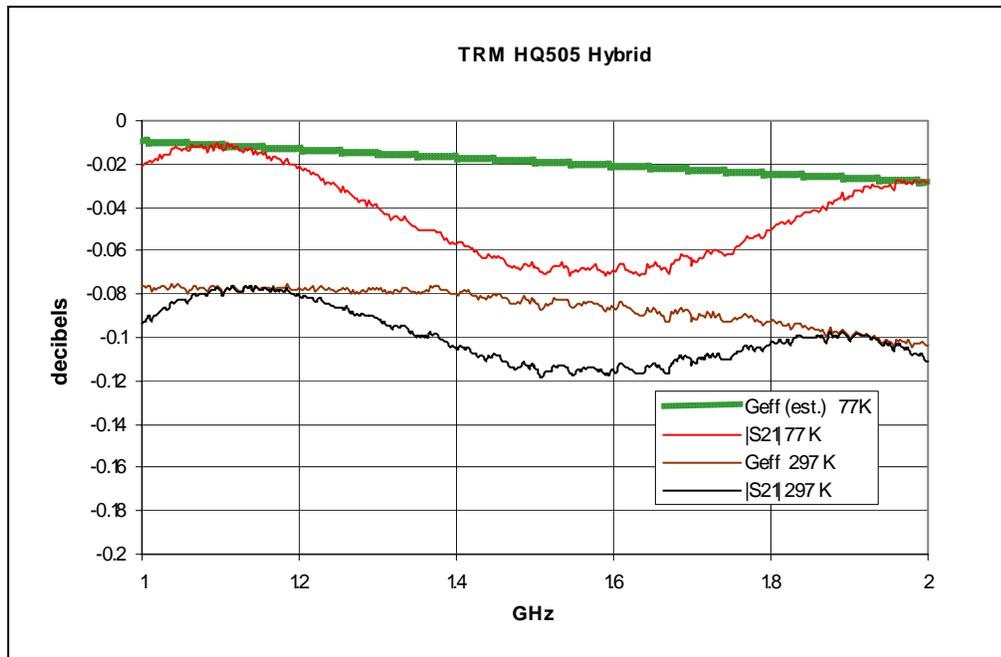
The bottom two traces are room temperature measurements. The lower is  $|S_{21}|$  and the one above it is  $g_{\text{eff}}$  (from S11 and S21 data).
