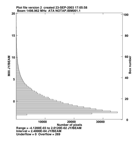
Figure 3: The histogram of the ATA configuration (version Q8A\_2W) side lobes inside of the ATA antenna primary beam. Natural weighting was used to create the PSF function. The PSF function has not been multiplied by the antenna primary beam. The peak side lobe is  $\sim 2\%$ . RMS of side lobes is  $\sim 0.27\%$ .
