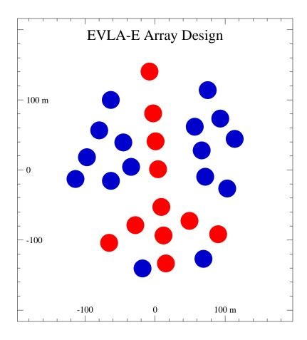
Figure 1: The EVLA E - configuration. The size of the dots shows the antenna diameter of 25 meters. The red antennas are on existing (D-configuration) pads. The blue dots mark locations of the proposed new pads.
