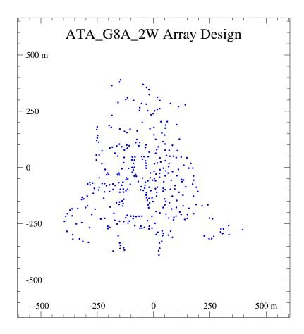
Figure 2: The ATA configuration (version Q8A $_2$ W). The size of the dots shows the antenna diameter of 6.1 meters.
