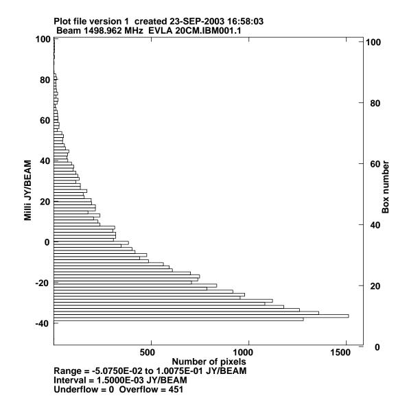
Figure 4: The histogram of the E-EVLA configuration side lobes inside of the EVLA antenna primary beam. Natural weighting was used to create the PSF function. The PSF function has not been multiplied by the antenna primary beam. The peak side lobe is  $\sim 8\%$ . RMS of side lobes is  $\sim 2.3\%$ .
