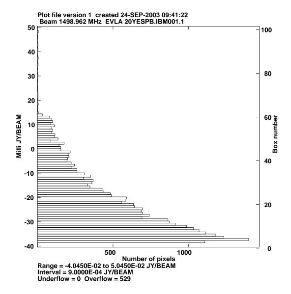
Figure 5: The histogram of the E-EVLA configuration side lobes inside of the EVLA antenna primary beam. Natural weighting was used to create the PSF function. The E-EVLA configuration was designed minimizing the product of the PSF and primary beam functions. Here the PSF function has been multiplied by the antenna primary beam. The peak side lobe is  $\sim 3\%$ . RMS of side lobes is  $\sim 1.2\%$ .
