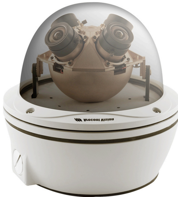
Figure 14. The all-sky camera. Four wide-angle lenses allow full hemispheric coverage above the site.
