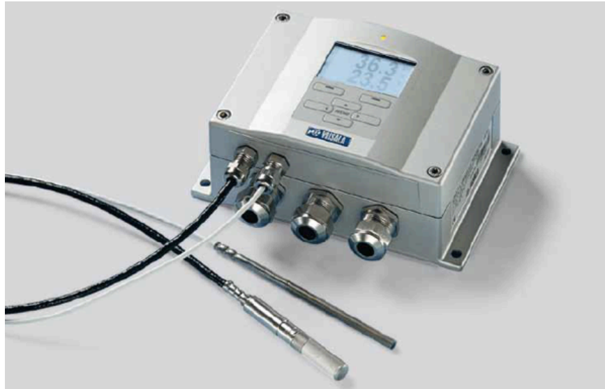
Figure 6. The Vaisala HMT337 relative humidity probe and transmitter. The heater is the black rod attached to the transmitter by the white wire. Note that the HMT333 unit is a duplicate of this, but without the heated probe.
