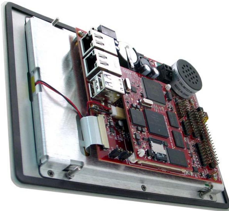
Figure 5 - Embedded Touch Panel Computer
