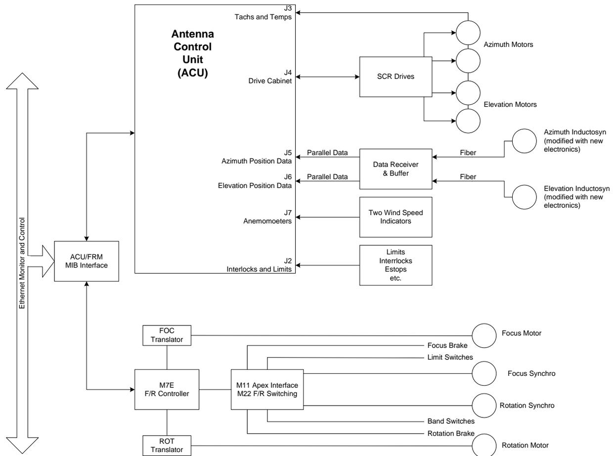
Figure 1 - Simplified Control System Block Diagram
