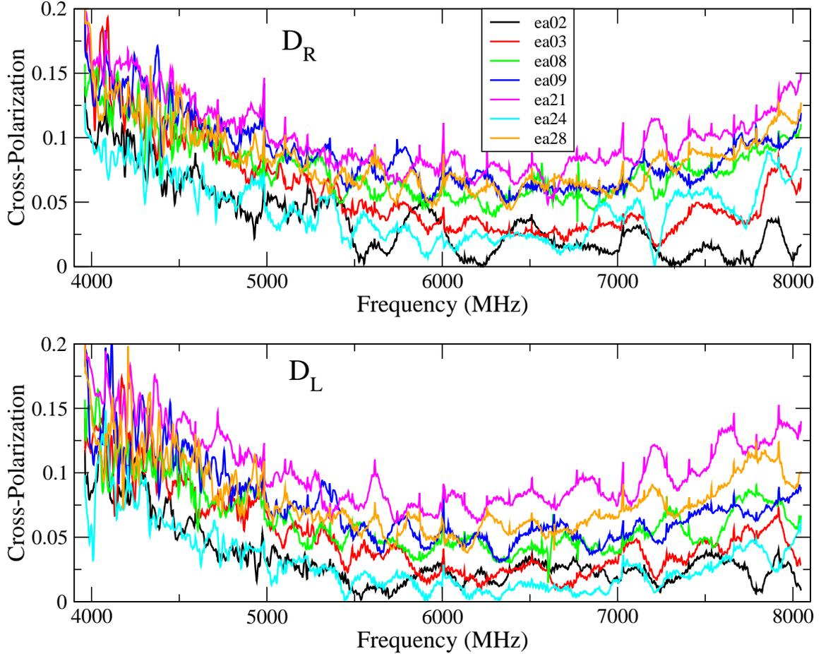
Figure 4: Cross-Polarization Amplitudes for seven antennas outfitted with the old quadrature hybrids at C-band.
