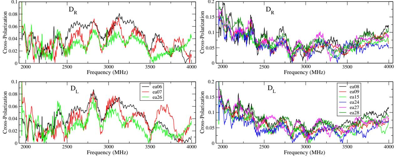
Figure 2: (Left) The cross-polarization amplitudes at S-band for three antennas outfitted with new design quadrature hybrids. (Right) The cross-polarization amplitudes for the old design hybrids. Note the change of scale – the old design is notably poorer than the new over the entire frequency range.
