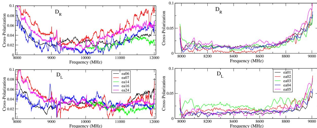
Figure 1: (Left) Cross-polarization amplitudes for the five antennas outfitted at X-band with the new wide-band polarizers. Most meet the 5% requirement over most of the band. (Right) The cross-polarization amplitudes for five of the old design polarizers. These narrow-band systems show much lower cross-polarization over their design bandwidth.
