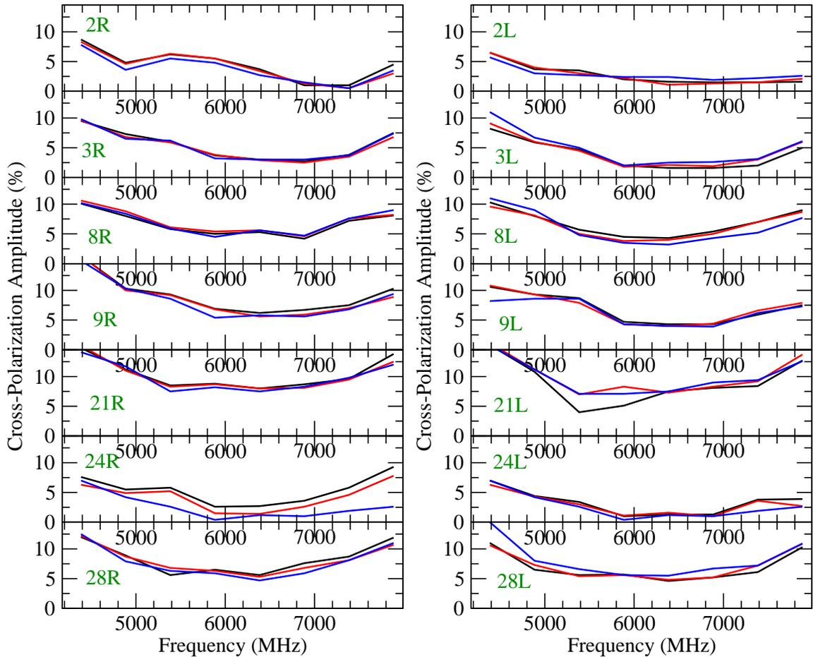
Figure 5: The change in C-Band cross-polarization for the seven antennas that have had wideband feeds since April 2009. The April 2009 results are shown in black, the January 2010 in red, and the new March 2011 in blue. For nearly all antennas, the change in cross-polarization over the two-year period is not more than a few tenths of one percent.
