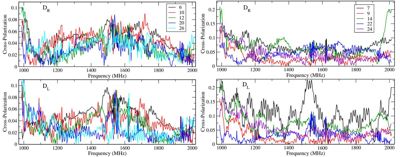
Figure 3: (Left) Cross-Polarization Amplitudes at L-band for five antennas outfitted with new design low-temperature quadrature hybrids. (Right) The results for five antennas with old-style. Note the change in scale. The new style provides better performance overall.
