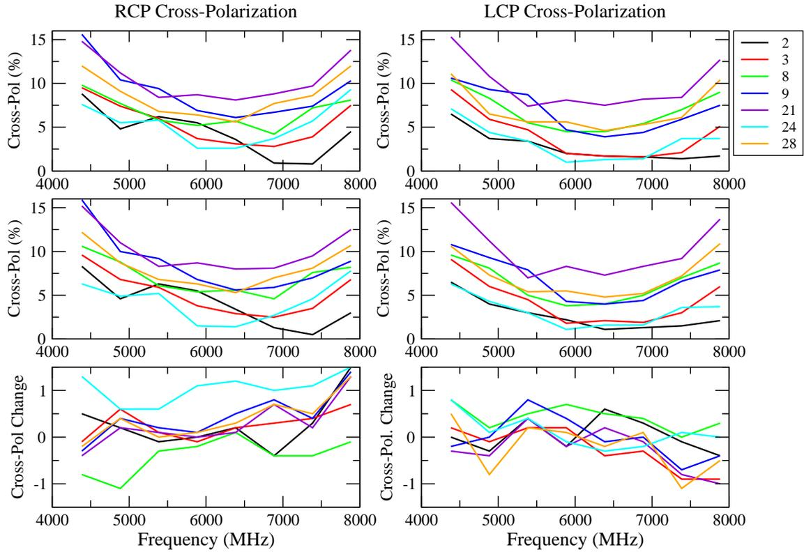
Figure 4: The C-band antenna polarizations  $|D_r|$  (left) and  $|D_l^*|$ . The top row shows the cross-polarization in April 2009, the middle row in January 2010. The difference is shown in the bottom row.
