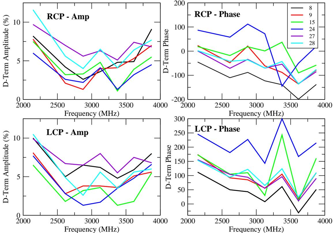
Figure 2: The S-band antenna cross-polarizations for the six EVLA antennas equipped with modern wideband receivers and polarizers. The LCP-Phase is negated.
