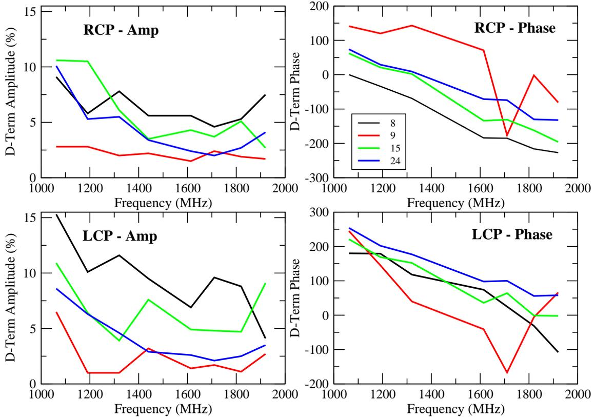
Figure 1: The L-band antenna cross-polarizations for the four EVLA antennas equipped with modern wideband receivers and polarizers. Note that the LCP-Phase plot has been negated, to permit easier comparison to the RCP-Phase.
