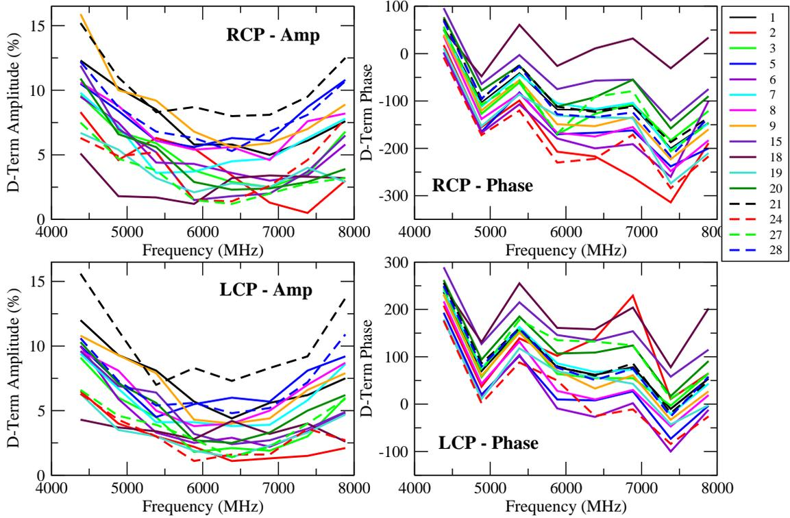
Figure 3: The C-band polarizations for the 16 EVLA antennas equipped with modern wideband receivers and polarizers. The LCP-Phase is negated.
