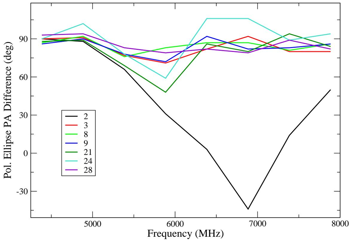
Figure 4: Showing the orthogonality of the EVLA antenna polarization ellipses. Except for antenna 2 (whose polarization at the higher frequencies is very low), the differences are close to 90 degrees, enabling acceptably low leakages in the cross-polarization baseline-based correlations.
