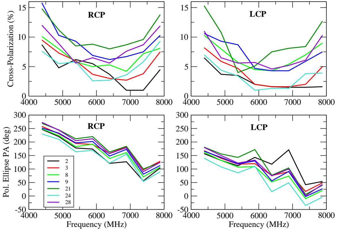
Figure 3: The upper panels shows the absolute cross-polarizations for all seven functioning EVLA antennas equipped with wide-band OMTs for RCP (left) and LCP (right). The lower panel shows the orientations of the polarization ellipses. The differences between RCP and LCP are close to 90 degrees for all antennas.
