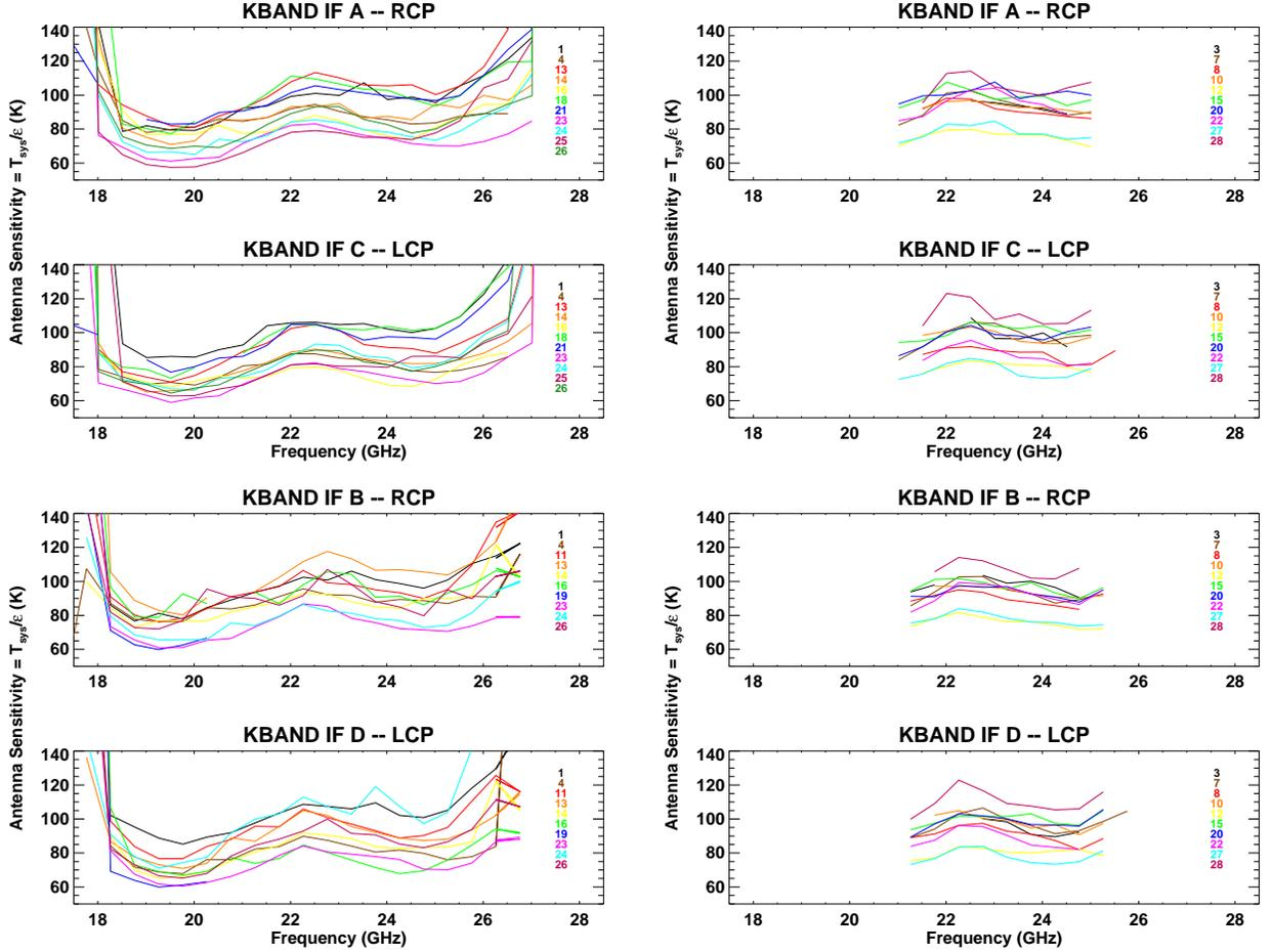
Figure 1: K-band antenna sensitivities. EVLA antennas (left) and VLA antennas (right) for all IF's and polarizations.
