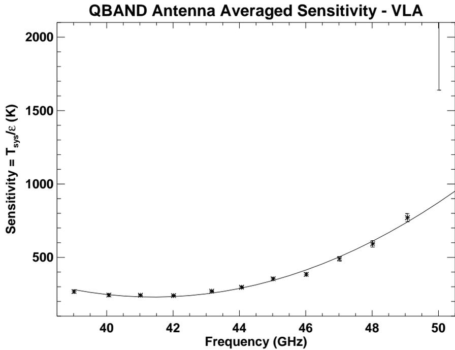
Figure 5: Q-band antenna averaged sensitivity values for the VLA antennas and the best-fit curve.
