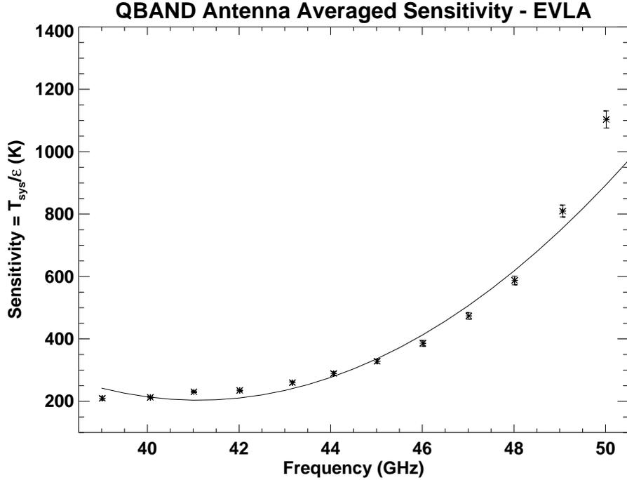
Figure 6: Q-band antenna averaged sensitivity values for the EVLA antennas and the best-fit curve.
