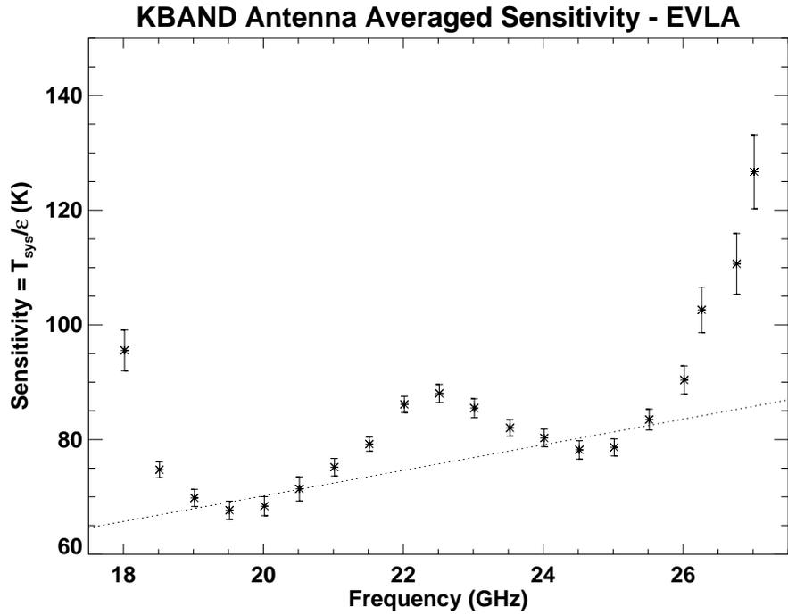
Figure 4: K-band antenna averaged sensitivity values for the EVLA antennas and the best-fit straight line curve. The best-fit line was produced by neglecting the region of the water line and the edges of the band. The water line reduces the sensitivity by approximately 10 K.
