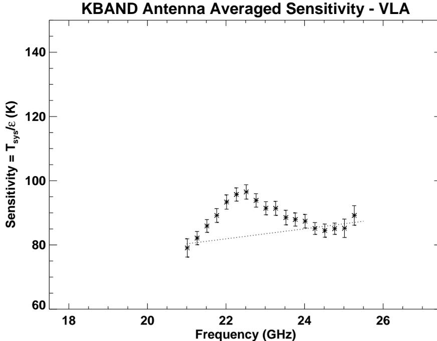
Figure 3: K-band antenna averaged sensitivity values for the VLA antennas and the best-fit straight line curve. The best-fit line was produced by neglecting the region of the water line. The water line reduces the sensitivity by approximately 10 K.
