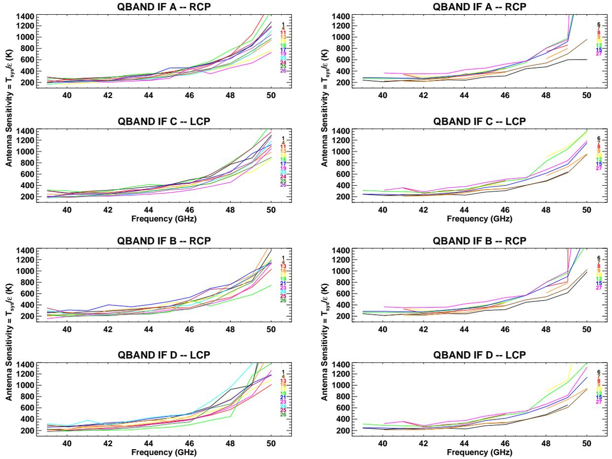
Figure 2: Q-band antenna sensitivities. EVLA antennas (left) and VLA antennas (right) for all IF's and polarizations.
