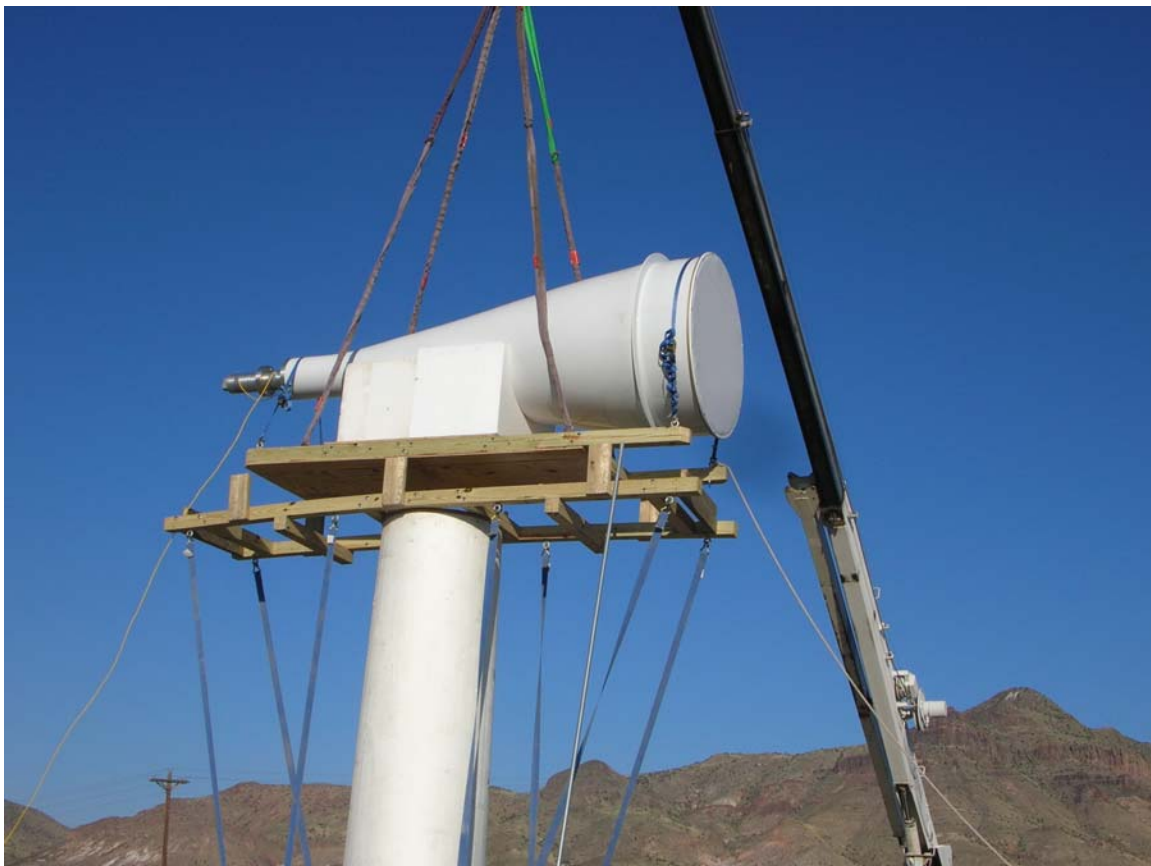
Figure 2. Range testing of S-band feed horn at OATR
