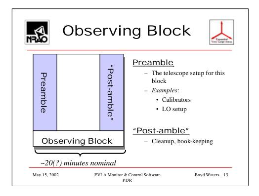
20 minutes is a typical calibration duty cycle. But the blocks can vary in size.
