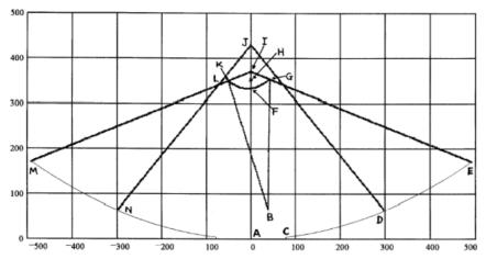
• Subreflector subtends 18 deg. Feed aperture is 7 wavelengths. Feed is large at L Band.
