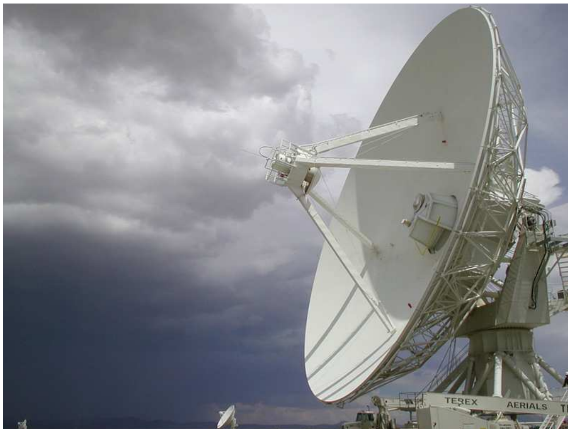
Figure A.1: The EVLA test antenna (VLA antenna #13) with its new feed cone installed in the middle of the reflector. This antenna is positioned on the VLA Master Pad for testing.
