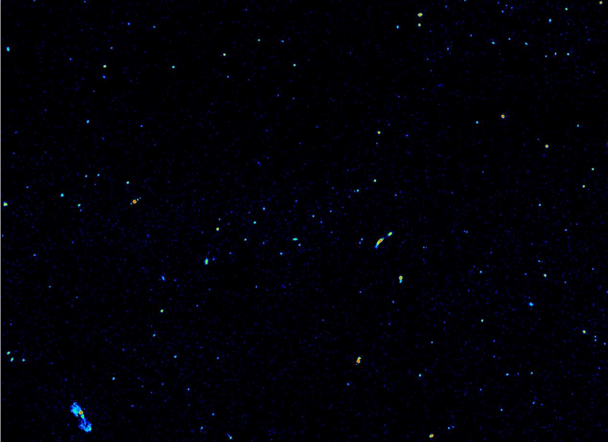
Figure 3.11: A 10.6 \times 7.7 arcmin 2 section of a deep ( \sim 120 hour) 1.4 GHz VLA image (rms noise \sim 3 \mu\text{Jy}/\text{beam} ); the resolution is \sim 1.5 arcsec, and the image shown is roughly a tenth of the full field-of-view. Such images will become routine with the increased sensitivity provided by the first phase of the EVLA Project. The New Mexico Array however will be able to actually image all these sources, providing \sim 10 beams across each source. This means that each of the pin-pricks in the current image will be resolved at roughly the level of the the extended, double-lobed source seen here in the southeast corner, aiding enormously in distinguishing AGN from starburst emission. Courtesy F. Owen (2003).
