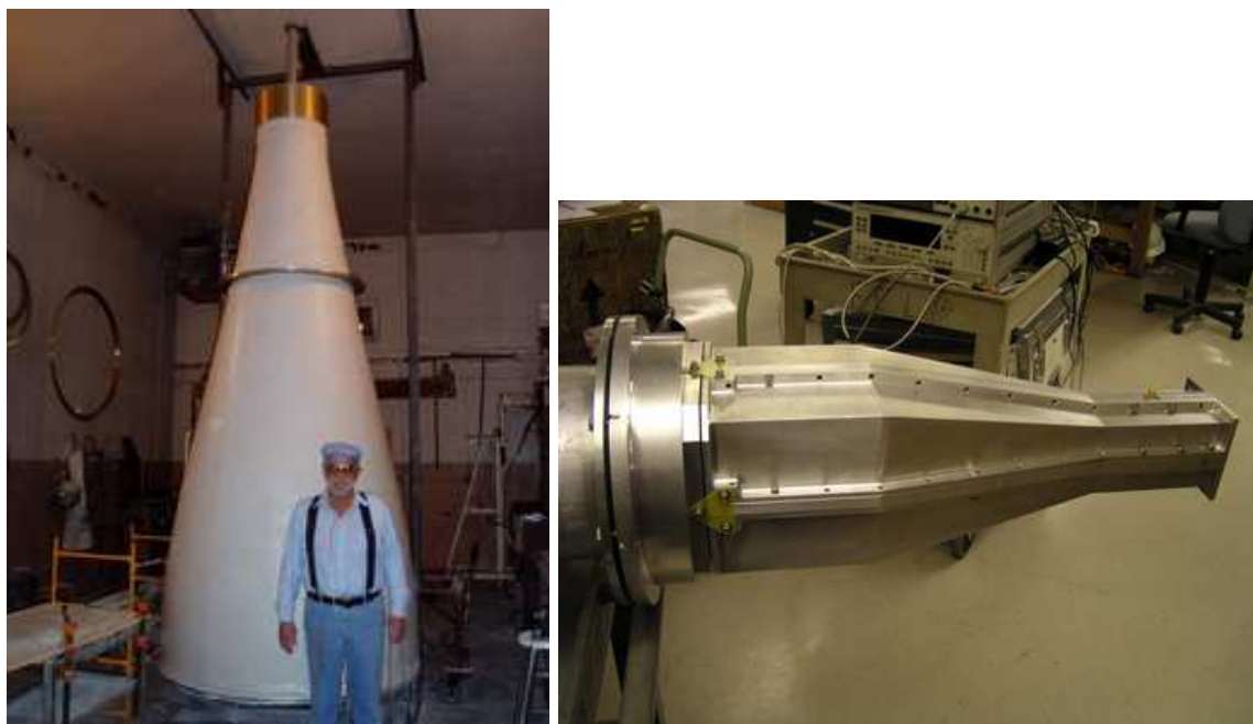
Figure A.2: Prototypes of the 1-2 GHz band feed horn (left) and polarizer (right). These are scheduled to be outfitted on the EVLA test antenna for testing in April 2004.
