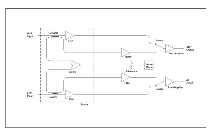
For source temperatures at the lower end of the solar range, the receiver temperature may not be negligible, and the assumption that all antennas have the same system temperature will not be valid. For this reason, each solar receiver will need its own solar noise calibration system. Since this consists mainly of the substitution of a controllable attenuator for a fixed one, the cost per receiver is small.
