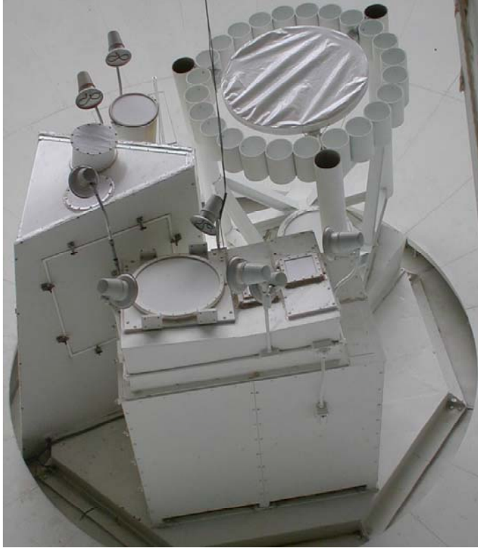
Figure 2 - VLA Vertex with K/Q Feed Cone Segment
