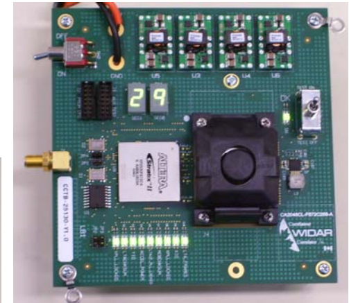
Test board for WIDAR correlator chip
