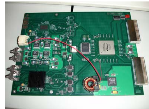
Prototype 3-bit, 4Gsps sampler
