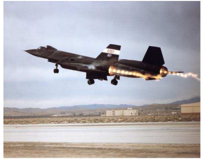
Figure 7: Example of internal shocks in a collimated supersonic jet due to a sudden drop in external pressure. The fact that the SR-71 is airborne shows that the internal shocks have little effect on the propagation and energy flux of the jet.
