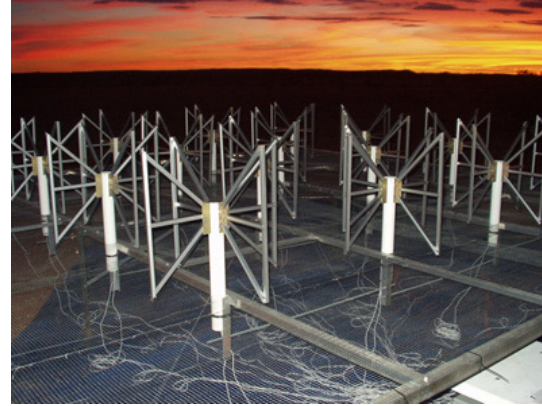
MWA 80-300 MHz. Steered by phasing fixed elements
