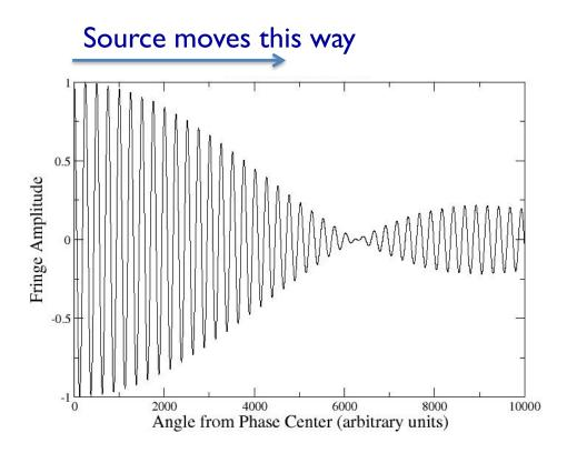
Maintaining phase stability requires much faster tracking than maintaining amplitude. The process is much easier if the phase adjustment can be done independently of delay.
