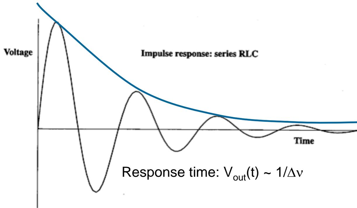
Response of RLC (tuned) filter of bandwidth  $\Delta\nu$  to impulse  $V(t) = \delta(t)$ : decay time ('ringing')  $\sim 1/\Delta\nu$
