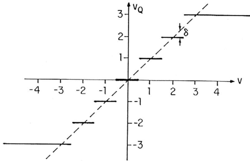
Figure 4-6. An example of a quantizer transfer function (solid lines); this quantizer has seven levels. The dashed line is the line defined by  $v_q = v$ , and the difference between it and the transfer function is the quantization noise,  $\delta$ .
