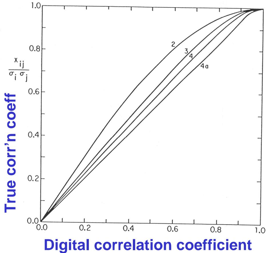
Figure 4-7. Quantization correction functions for various quantizations. In each case the signal powers are set for maximum signal-to-noise ratio. The curves are labeled according to the number of quantization levels; 4a uses a simplified multiplier (see Cooper, 1970).
