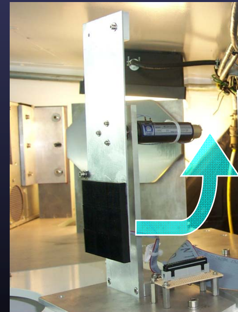
SMA calibration load swings in and out of beam
