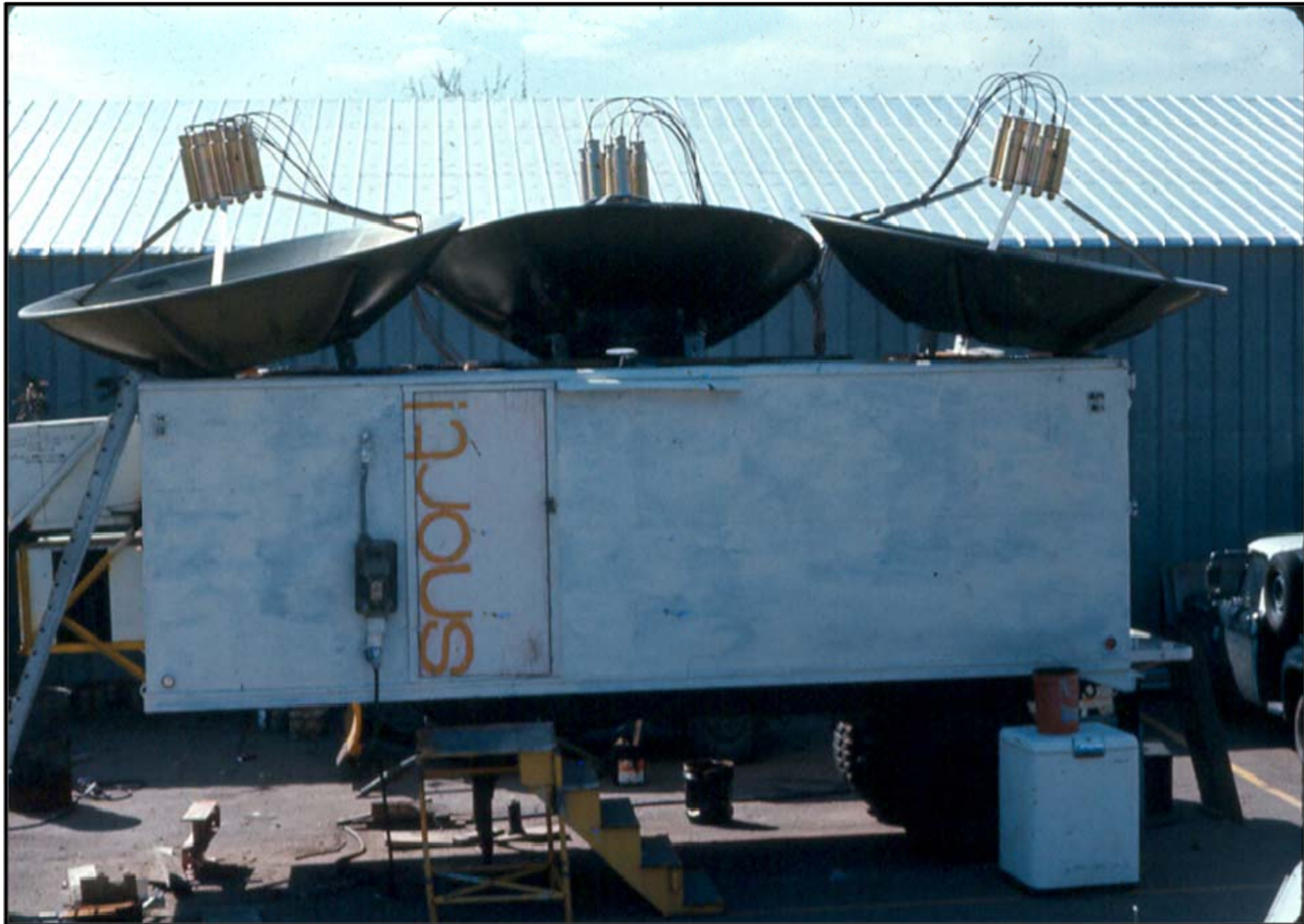
A close-up picture of the SNORT experiment's trailer and its three 7-beam telescopes which yielded 21 separate beams on the sky searching for a microwave pulse from an exploding star (photo courtesy of Bruce Blevins)
