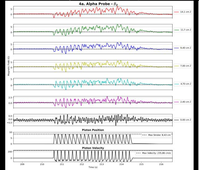
$f_{in}=f_{out}=10.5$  Hz,  $f_{jet}{\sim}5.5$  Hz,  $f_{sample}=2000$  Hz  $Rm_{\omega}=0$ ,  $Rm_{\alpha,twist}=2.67$ ,  $Rm_{\alpha,expand}=3.92$
