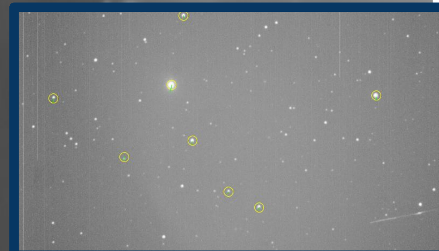
Stars are automatically selected in order to determine rotation and/or translational motion.
