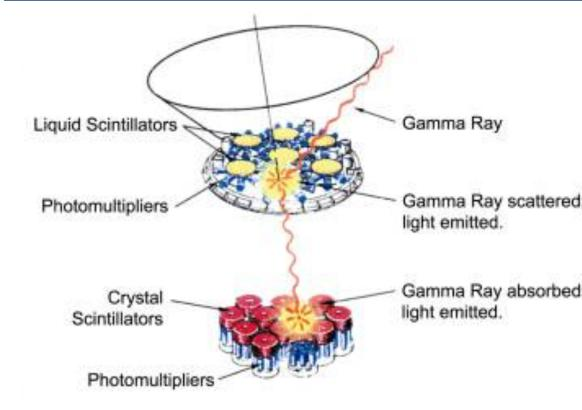
A Compton telescope takes advantage of Compton scattering to form images in the difficult MeV gamma-ray range. The only successful astronomical Compton telescope, COMPTEL, relied on time-of-flight (ToF) measurements between two scintillator detector layers to reject background.
