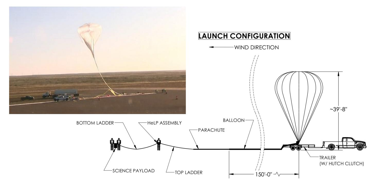
Los Alamos is currently developing a dedicated small balloon platform for use with CSBF's hand-launch capability. The inaugural flight is planned for Fall of 2021 from Fort Sumner, where we will test an advanced imaging gamma-ray detector made of cadmium-zinc-telluride (CZT) in collaboration with the University of Michigan:
