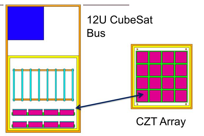
We modeled a payload of 32 cadmium-zinctelluride (CZT) gamma-ray spectrometers flown in a 12U CubeSat bus  $(20 \times 20 \times 30 \text{ cm}^3)$  using MCNP.
