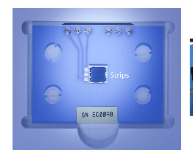
The SCDDs are being developed at Southwest Research Institute. Each is 4.5 ×  $4.5 \times 0.5 \text{ mm}^3$  and patterned with 3 readout strips per side. A custom readout board provides position, energy, and timing signals.
