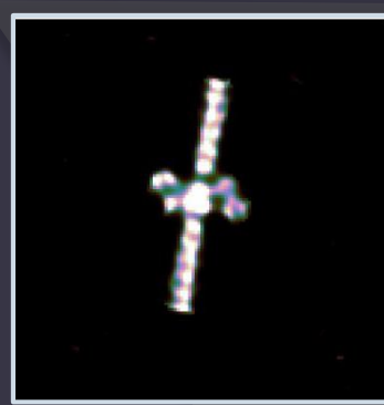
Simulated image Direct-TV Satellite #9 accomplished in 2 hours using 10-element MROI plus 2.4m scope with aperture masking
