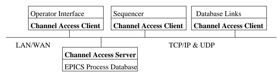
Client: Provides read/write connections to any subsystem on the network with a channel access server
