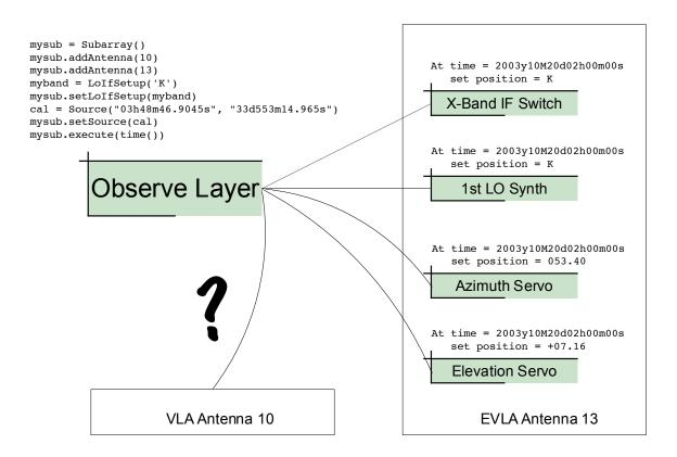
The current Observe Layer communicates directly with EVLA antenna subcomponents. VLA antennas contain different subcomponents so they cannot be controlled by this system without significant changes to it.
