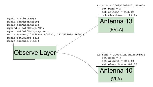
The Observe Layer should communicate with the AMCS Antenna Objects not the antenna subcomponents.
