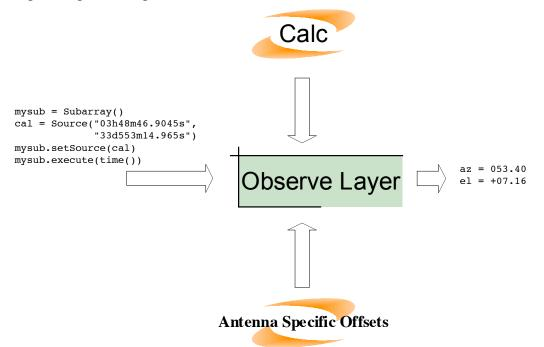
The Observe Layer, using inputs from CALC and Antenna Offsets Tables, converts observation program syntax and values into discreet state values that the system understands.
