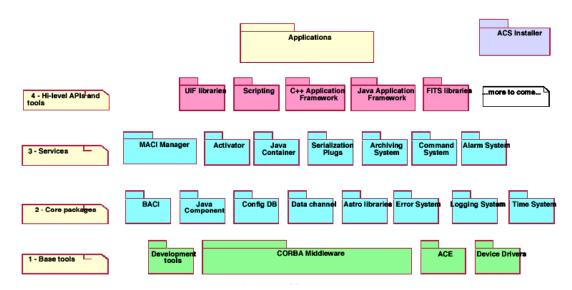
The core layer contains the system 'components' which are similar to the EVLA software 'Device'. This is the software that represents the physical system that is to be controlled and monitored.
