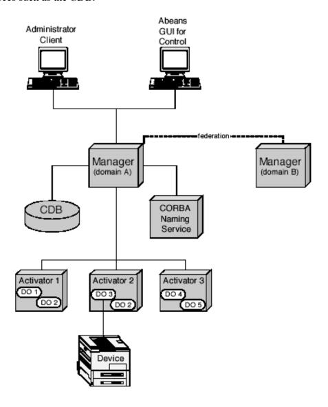
When a distributed processor comes online, it starts its Activator (or Java Container) that, in turn, establishes a connection via CORBA to the Manager. The Manager checks to see which DO's (or Java Components) are hosted by the Activator and orders them brought to life.
