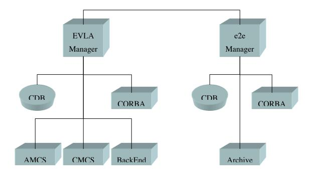
This would have the advantage that e2e and the rest of the outside world would see the EVLA via ACS. The EVLA would consist of only three ACS components, the AMCS, CMCS and Correlator Backend.
