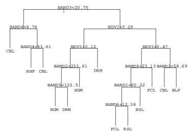
**Fig. 2.** Binary decision tree showing the levels of different spectral characteristics at which vegetation classes separate.
