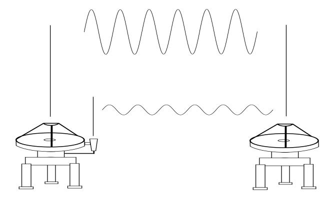
Figure 1: The overall arrangement for the gain measurement. Either the standard gain horn or the regular feed can be connected to the receiver of the antenna on the left.
