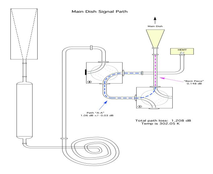
Figure 2: The circuit showing how either the standard horn or the feed may be switched to the receiver.
